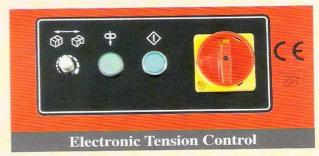
External adjustment of strap tension by the simple turn of a dial.
